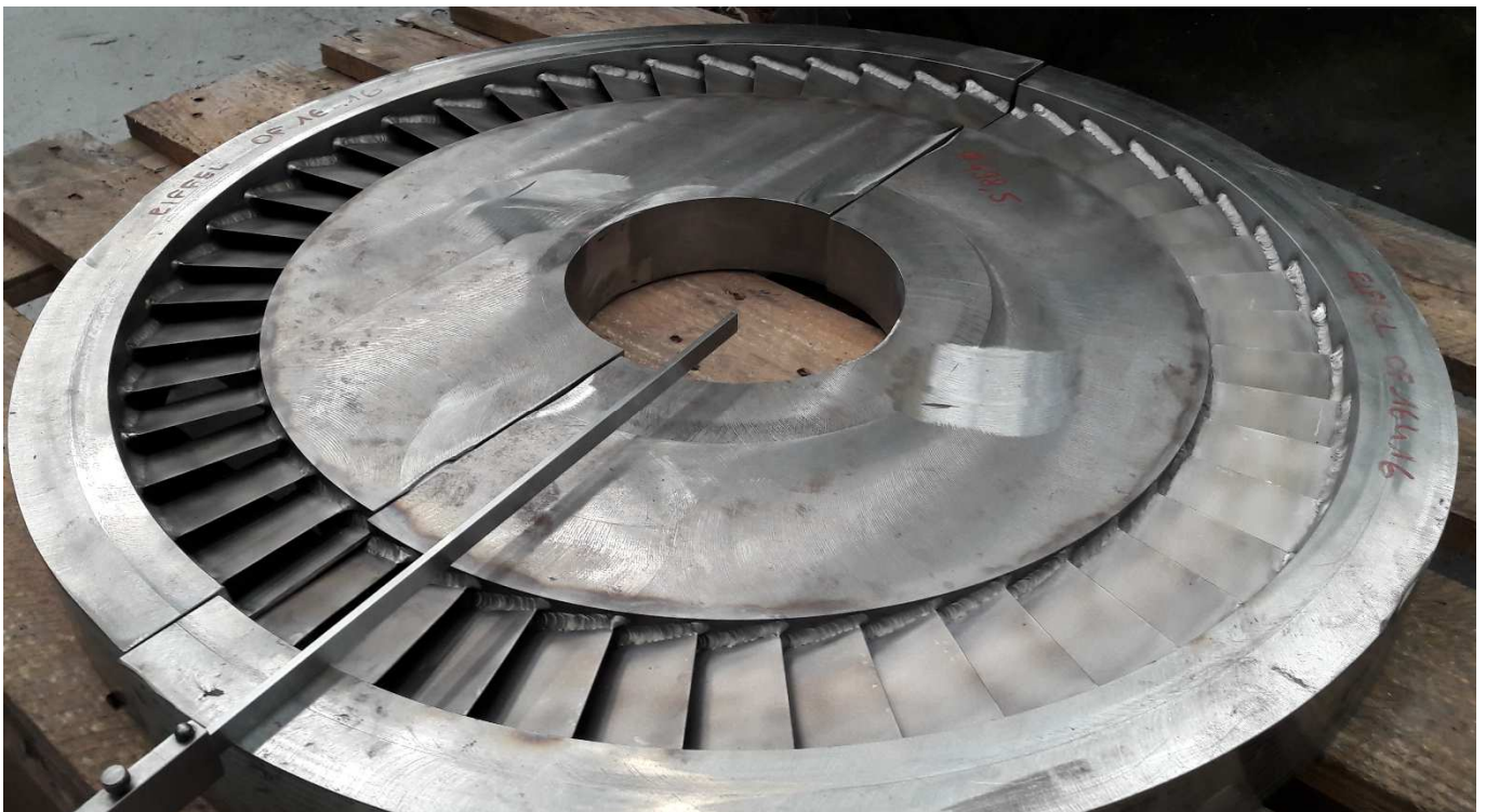
DIAPHRAGME : PLANS DE JOINT, PIETAGE, ØEXT&FACE (25CD4S)
